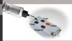
S-L-O-W-L-Y drip ink onto the felt pad showing in the outlet port. The ink will be absorbed quickly into the cartridge.
