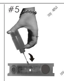
Push the needle all the way in and very slowly inject the ink into the sponge as you slowly pull the needle upwards
