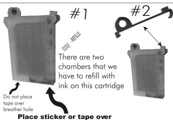
Remove the cap With a flat knife or small screw driver by placing between the cap and the cartridge body and then twisting to lever the cap upwards.
