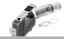
S-l-o-w-l-y and gently squeeze the ink refill bottle to force ink into the reservoir until it is almost full.
