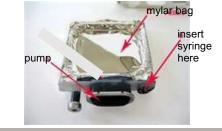
Remove the plunger from the syringe. Put the point of the syringe over the filling hole and blow into the open end (where the plunger was). This expands the mylar bag inside the cartridge so it will accept the ink.
