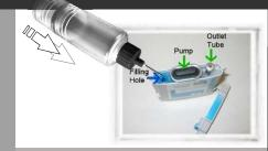
S-I-o-w-I-y squeeze the ink refill bottle to force ink into the reservoir - about half the bottle should go in.
