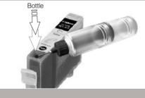
S-I-o-w-I-y and gently squeeze the ink refill bottle to force ink into the reservoir until it is almost full.
