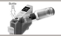
Insert the refill needle into the filling hole. Angle the needle toward the ink outlet hole at the bottom of the cartridge and push down as far as possible.
