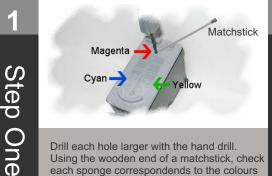
Drill each hole larger with the hand drill. Using the wooden end of a matchstick, check each sponge correspondends to the colours on this sheet BEFORE refilling.
